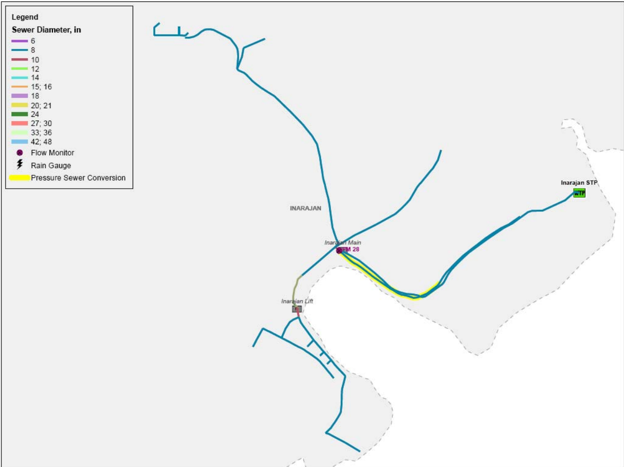
Figure 9-14 – Inarajan STP Pressure Sewer Upgrades
